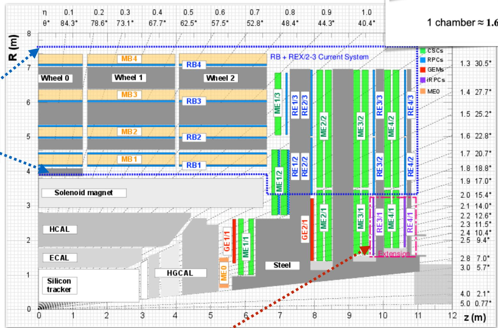
Extend the RPC coverage up to  $|\eta| = 2.4$  to increase redundancy in high eta region in stations 3 and 4. (72 iRPCs)
